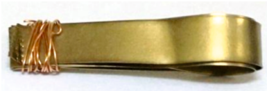
Fig.3: Deuterium loaded metallic titanium getter strips.
